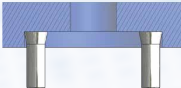
Messen eines Sacklochs Measuring of blind holes
