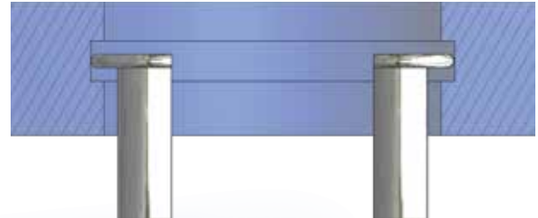
Messen einer Innennut Measuring of internal recesses
